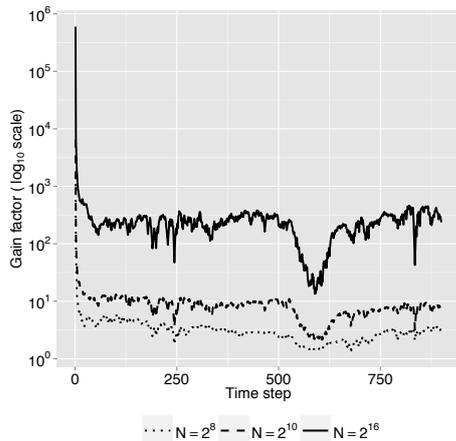
**Fig. 3.** Filtering of the state-space model (6): The plot gives the gain factor, defined as the  $\text{MSE}(\text{SMC})$  over  $\text{MSE}(\text{SQMC})$ , as a function of  $t$  for the estimation of  $\mathbb{E}[x_{1t}|\mathbf{y}_{0:t}]$ . The results are obtained from 100 independent runs of SMC and SQMC.
