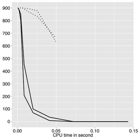
**Fig. 4.** Filtering of the state-space model (6): The plot gives the number of time steps  $t \in \{0, \dots, 899\}$  such that  $\text{MSE}(\hat{x}_{ti}) \geq 0.01^2 \text{Var}(x_{ti}|\mathbf{y}_{0:t})$  as a function of the CPU budget (average CPU time per iteration), where  $\hat{x}_{it}$  is either the SQMC (solid lines) or the SMC (dashed lines) estimate of  $\mathbb{E}[x_{ti}|\mathbf{y}_{0:t}]$ ,  $i = 1, 2$ . The results are obtained from 100 independent runs of SMC and SQMC.
